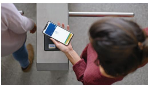
VSAM allows a chip to be introduced in the readers that is able to securely accept the NFC (Near Field Communication) technology found in EMV® payment cards and mobile devices, such as cell phones, bands, and watches. Its differential is that it accelerates implementation and lowers commercial deployment costs, since it does not require that the existing transportation card reading system be replaced.
